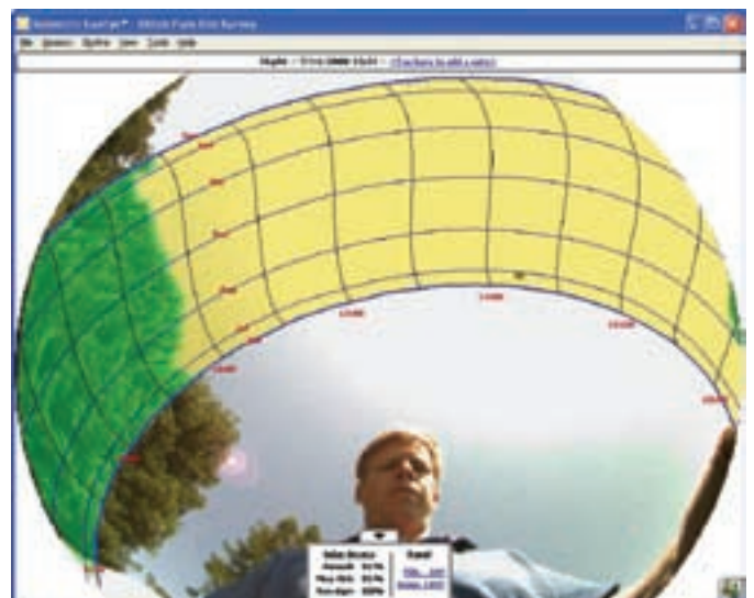
Image 1 Using a fish-eye lens, solar access measurements and computed results can be charted.
